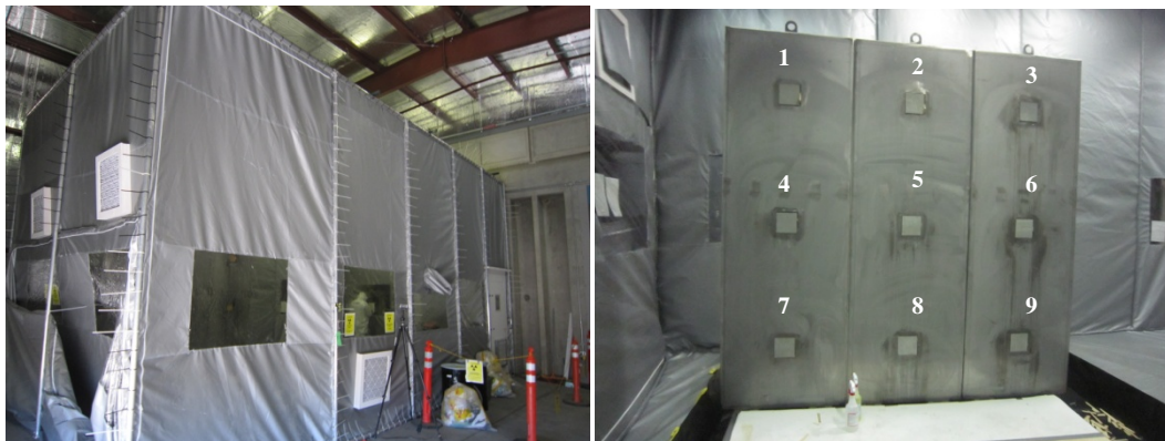
Figure 3-2. Containment tent: outer view (left) and inner view with test stand containing contaminated coupons with numbered coupon positions (right).
